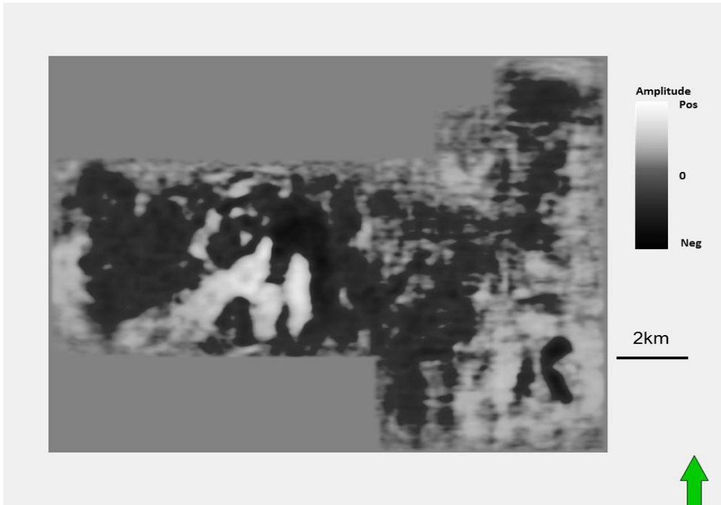
Figure 5.7. Time slice at t=0.6 s through stacked amplitude volumes conventional migration. The white block arrow indicates the footprint, which impedes the interpretation
