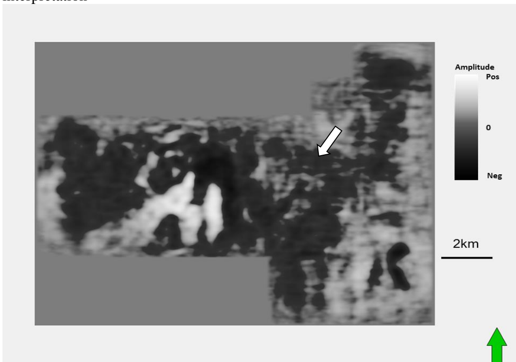
Figure 5.8. Time slice at t=0.6 s through stacked amplitude after two iterations of PLSM. The white block arrow indicates area where the footprint is attenuated.
