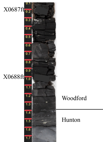
Figure 69: A piece of core showing the erosional unconformity between the Hunton Limestone and the overlying Woodford Shale.
