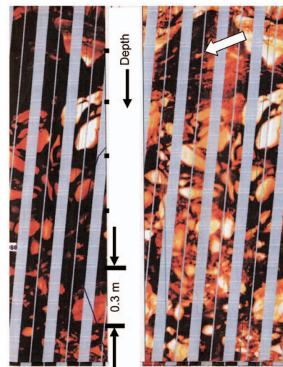
Figure 15. Resistivity-based image log showing karst breccia fabric, including rounded plus angular matrix-supported clasts and stratified fine sediment (white arrow). Location of well is indicated by arrow in Figure 12e; note that well location is not within a major collapse feature (data courtesy of Devon Energy).
