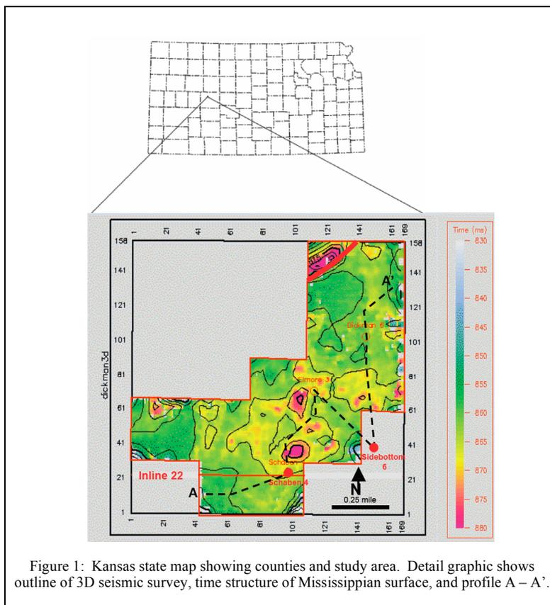
Figure 1: Kansas state map showing counties and study area. Detail graphic shows outline of 3D seismic survey, time structure of Mississippian surface, and profile A - A'.
