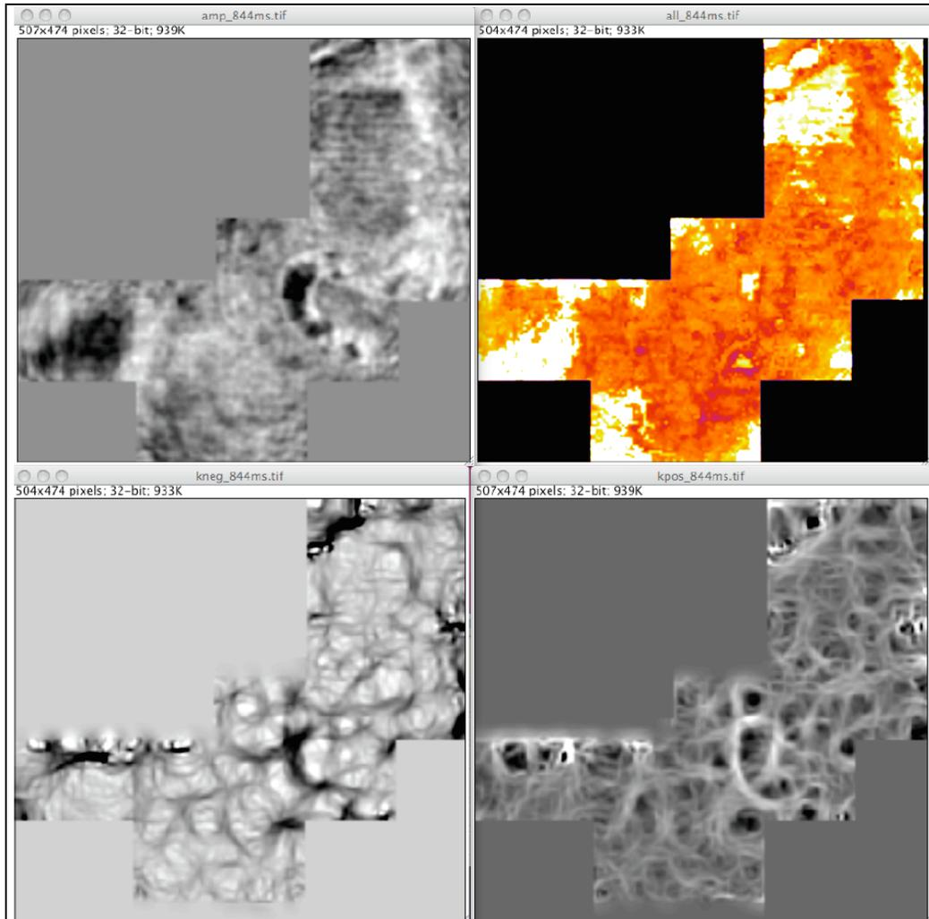
Figure 4: Selected seismic attributes from the 3D data at the Mississippian level (844 ms). Clockwise from upper right: Amplitude, impedance computed from full-range PSTM stack (orange to white is low to high value), negative curvature, and positive curvature. In all grayscale images, white is max positive and black is max negative. See Figure 1 for scale.
