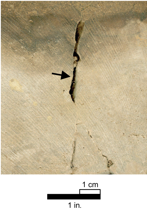
FIGURE 9. Core scan from 3.7 m (12 ft) below the top of the Mississippian in the Tilley 2 well. The black arrow indicates a small solution-enlarged vertical fracture in the Mississippian dolomite reservoir.
