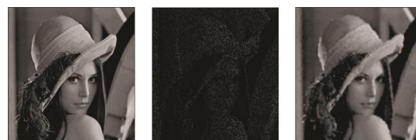
Figure 1: Interpolation of a sparsely, irregularly sampled image using normalized convolution. (Left) the famous image of "Lena". (Middle) A randomly sampled image containing only 10% pixels of the original image. (Right) Reconstructed image using normalized convolution.
