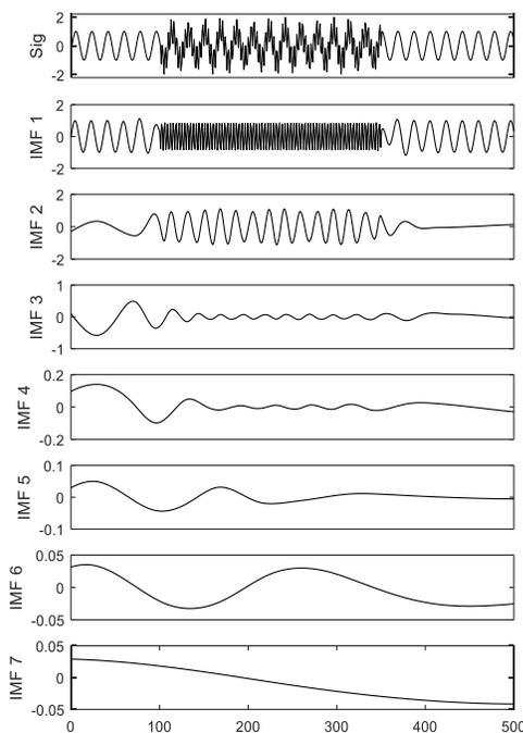
Figure 1: Decomposition of the artificially mixed signal by EMD.
