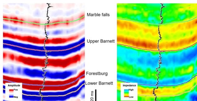
Figure 4: Field application. (Left) Seismic profile. (Right) Inverted seismic impedance.
