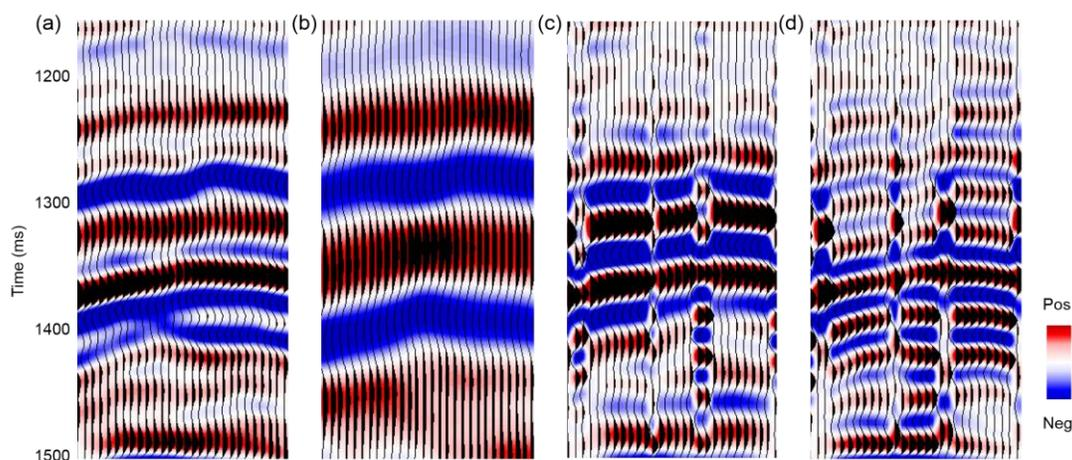
Figure 6: Example of traditional VMD. (a) Seismic and (b-d) different IMFs .
