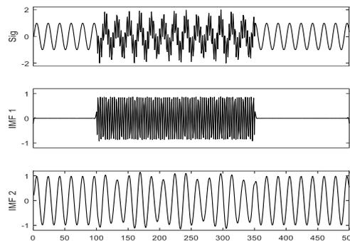
Figure 2: Decomposition of the artificially mixed signal by VMD.
