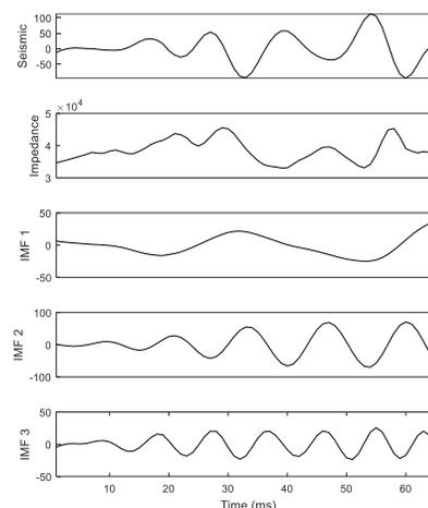
Figure 5: Seismic decomposition from VMD of Marble falls Limestone.
