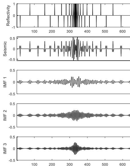
Figure 3: Normal-inverse cycle model test: reflectivity series, seismic and IMFs from VMD.
