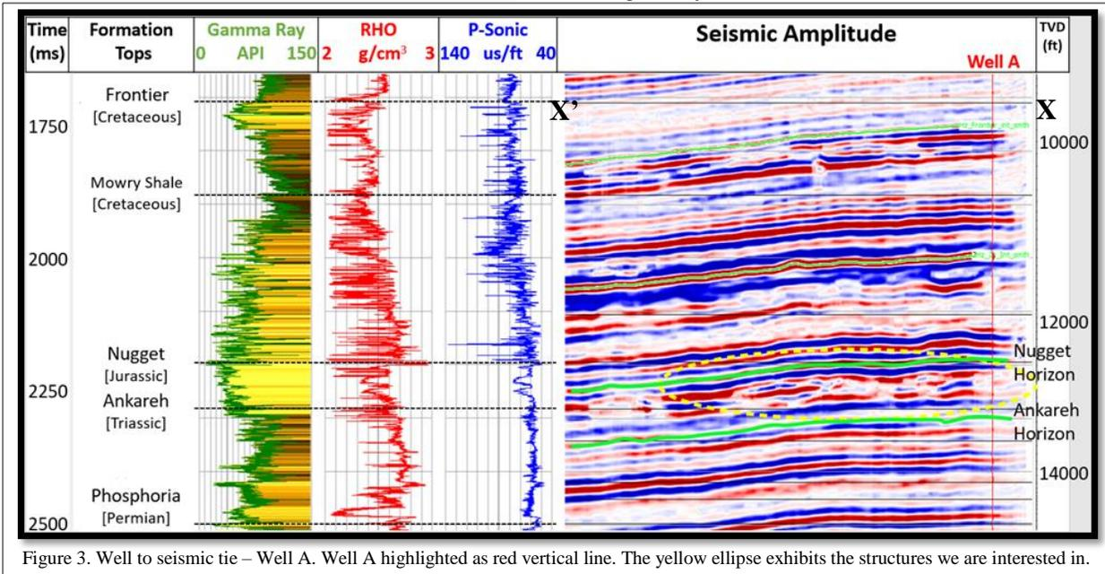
Figure 3. Well to seismic tie – Well A. Well A highlighted as red vertical line. The yellow ellipse exhibits the structures we are interested in.
