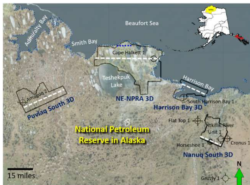
Figure 1. The study area in the NPRA, Alaska, with all 3D seismic surveys (outlined with black polygons) and wells (the black dots) used in this study. Four large 3D seismic surveys (Nanuq South 3D, Harrison Bay 3D, NE-NPRA 3D, and Puviaq South 3D) and several wells (Grizzly 1, Horseshoe 1, Itkillik River Unit 1, Cronus 1, Flat Top 1, South Harrison Bay 1, Cape Halkett 1, and Amaguq 2) with conventional and advanced petrophysical logs are available for this study.
