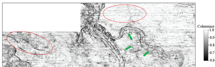
Figure 8. Multispectral coherence computed using six equally spaced CWT spectral voices (Figure 7), providing an image with less noise (especially the red circles) and clearer channel boundaries (especially the green arrows) than full-bandwidth coherence (Figure 5).
