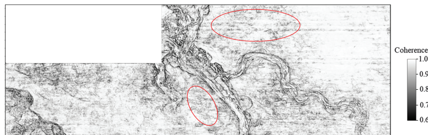
Figure 16. Multispectral coherence image computed using six spectral probes. It exhibits more balanced than the multispectral coherence images from other spectral decomposition methods but is noisier due to the equal weight for the noise in the shorter period components when we build the covariance matrix (the red circles).
