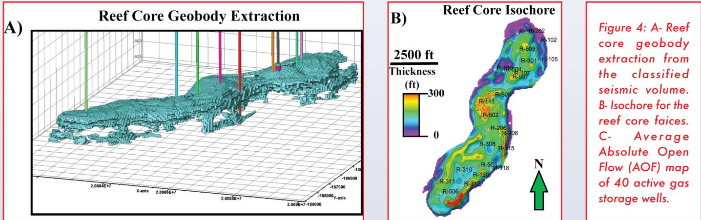
Figure 4: A- Reef core geobody extraction from the classified seismic volume. B- Isochore for the reef core faices. C- Average Absolute Open Flow (AOF) map of 40 active gas storage wells.
