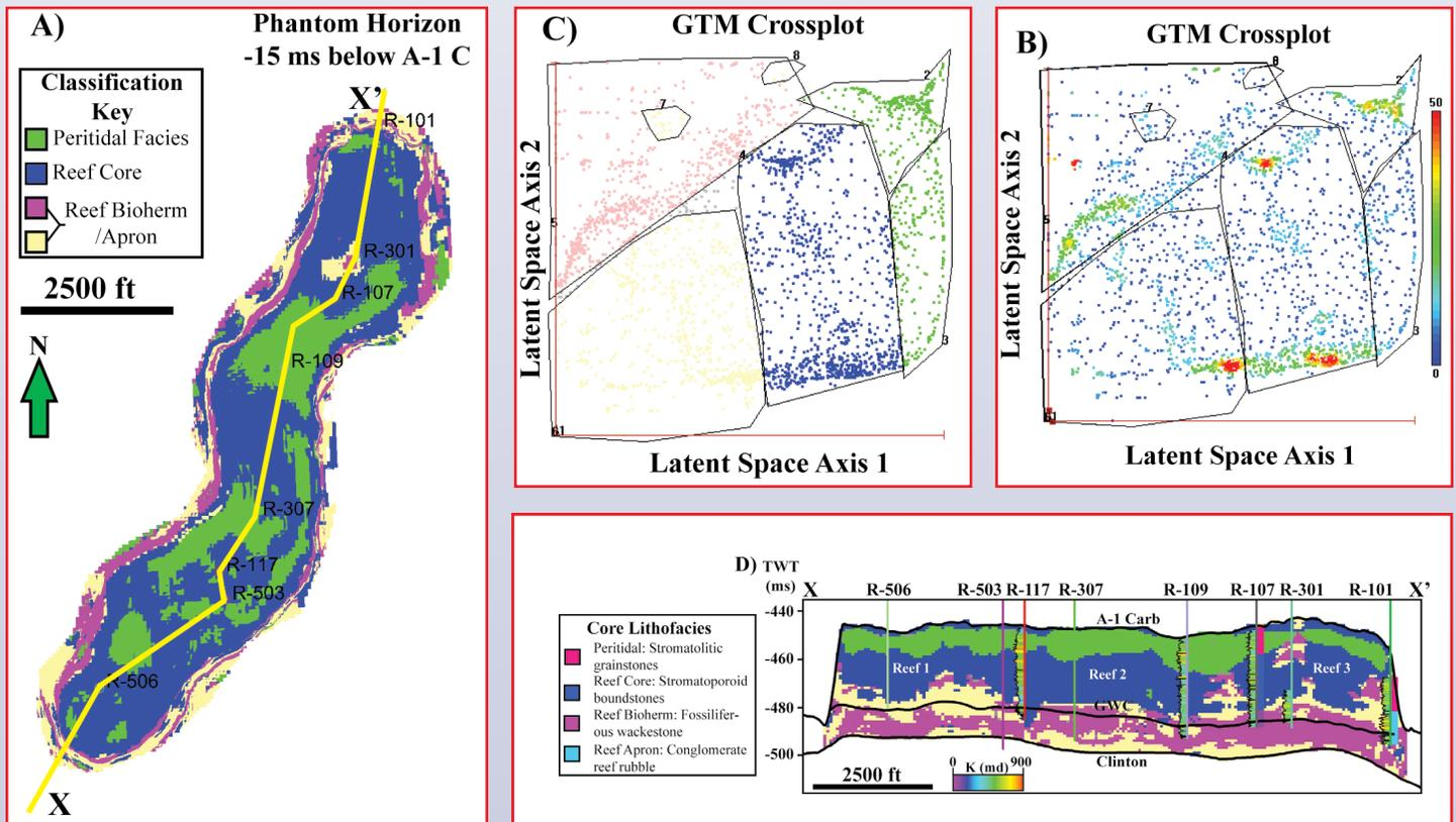
Figure 3: A- Phantom horizon 15 ms TWT below the A-1C horizon. B- GTM latent space axes cross plot with the data points colored by cluster density. The points represent the data shown in D. C- GTM latent space axes cross plot with the data points colored by class. D- Arbitrary cross section through the classified volume. Core-derived lithology and permeability logs are shown where available.
