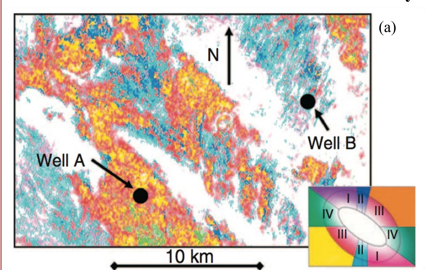
(a)Foster et al. (2010) discriminated depending on the class of AVO anomaly sands with good porosity (Well A) normally AVO class III represented by red and yellow colors from lower values of porosity (Well B) with AVO class II represented with blue color.
