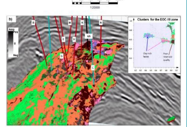
Facies classification from GTM for reservoir unit. (a) Seismic facies map 10 ms below top of EOC-10. Pie charts are proportional to daily average production for the first seven months. (b) 3D view of the volume probe containing clustering from GTM analysis. Insert crossplots are generated directly in the 2D latent space.
