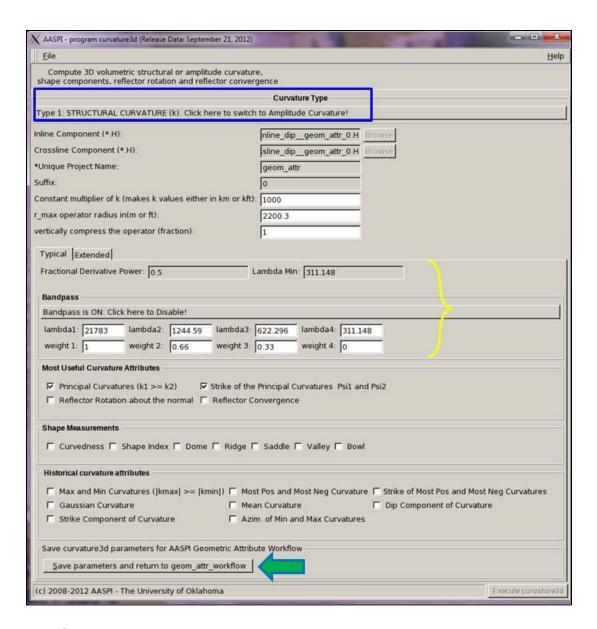
The GUI for curvature3d; the output from the imagefilt3d will be input to this program. Enter the proper parameters and then save and exit (*green arrow*). The parameter file get saved automatically as a curvature3d.parms file.
