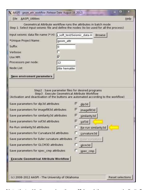
Note that with the saving the sof3d and the re-run similarity3d is activated. The re-run similarity calculates again the energy-ratio, Sobel-filter attributes taking in the PC or LUM filtered seismic dataset (output from the sof3d program). Thus it is sometimes better to re-run the similarity3d attributes so that the attributes are created on the filtered volume.
