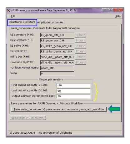
The GUI for euler\_curvature; the output from the curvature3d will be input to this program thus the button for euler\_curvature gets activated only after saving the curvature3d parameters. Enter the proper parameters and then save and exit (*green arrow*). The parameter file get saved automatically as a euler\_curvature.parms file.
