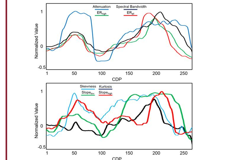
Fig 8: Seismic attenuation attributes between the pink and yellow horizon shown in Fig 6. Attenuation estimation using the central frequency shift (CFS) method, spectral bandwidth, energy reduction in full bands and high frequency bands, spectral slopes of low and high frequencies, skewness and kurtosis.
