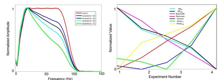
In the field, the wavelet may not always be the Ricker wavelet. After spectral balancing (bluing), the flat spectrum is usually expected. Fig 3 shows a synthetic example using Ormsby wavelet with corner frequency 10-20-80-100 Hz. The results show that most of the attributes still work.
