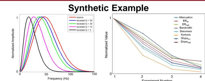
Figure 2 shows the normalized spectra of reference and attenuated signal. Note that when attenuation is stronger, the peak frequency is smaller, and more high frequency energy attenuated. Results of attenuation attributes associated with different Q values are also displayed. Because we want to know the relative attenuation relationship, all values are shown in the normalized way. It is clear that every attributes has a good correspondence with the attenuation factor.
