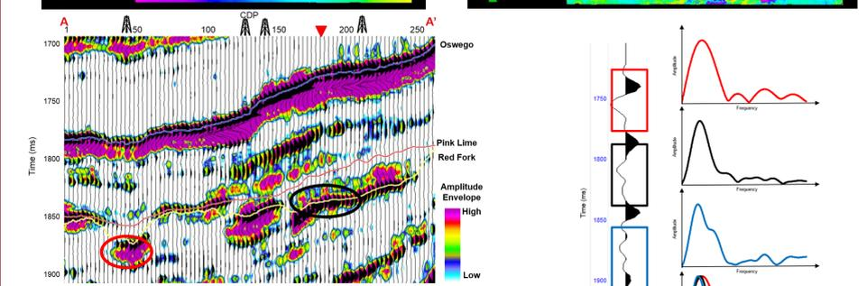
Fig 7: Single trace example (extracted from CDP 170, denoted as a red triangle in Fig 6) of seismic spectral changes with increasing depth.
