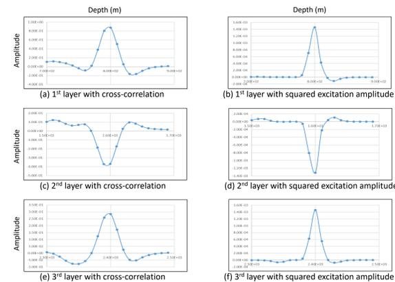
Figure 4. Comparison of migration resolution of the multi-reflector model
