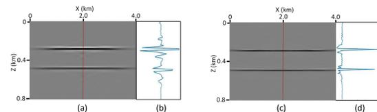
Figure 1. Least-squares PSPI migration of synthetic data. The least-squares migration (c) has better imaging quality over conventional migration (a). (b) and (d) are the single traces extracted from the center location.
