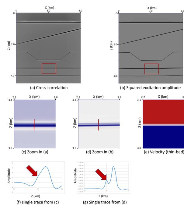
Figure 8. Numerical test of thin-bed model, note the thin bed indicator by the arrow.
