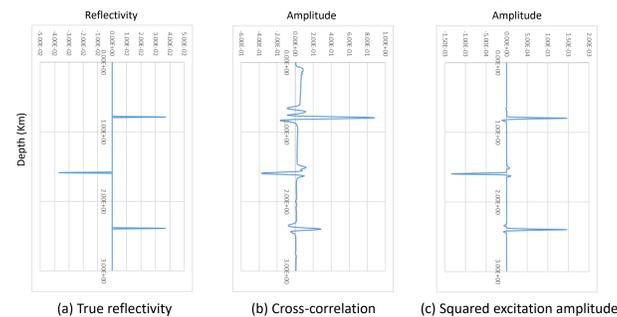
Figure 6. Comparison of amplitude preservation with single trace images
