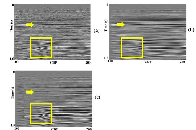
Figure 8: (a) Original seismic data. (b) Filtered data after applying the workflow. (c) Workflow applied to the data after flattening on the dipping reflector.
