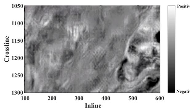
Figure 5: A horizon slice along the top PaloPinto through amplitude volume after filtering.
