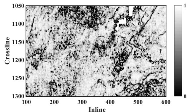
Figure 6: A horizon slice along the top PaloPinto through coherence volume.
