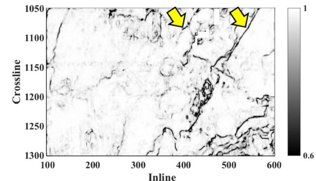
Figure 7: A horizon slice along the top PaloPinto through coherence volume after filtering.
