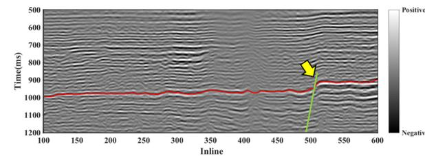
Figure 3: Crossline 1090 through the north Texas seismic data with PaloPinto horizon picked on the data. The yellow arrow indicates the fault that cuts through the horizon.
