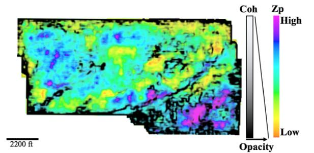
Figure 6: The impedance computed on 5D interpolated data co-rendered with the coherence computed on the original data. Note the coherence anomaly seems to delineate the high impedance (magenta) anomaly in the SE part of the image.
