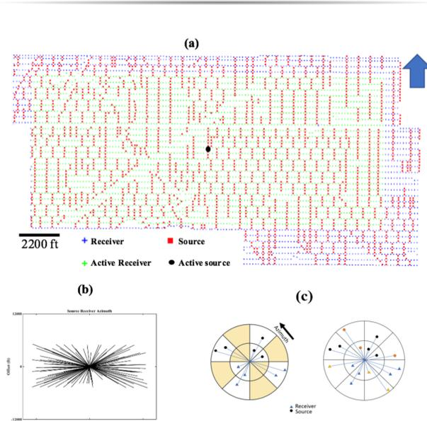
Figure 2: (a) A map showing the survey acquisition geometry. (b) Spider diagram for a common midpoint gather. Notice the survey has longer offsets in the E-W direction than in the N-S direction and hence is a narrow azimuth. (c) cartoon showing the annulus sector binning of a common midpoint gather with two offset and four azimuthal sector bins for (left) data before and (right) after 5D interpolation.
