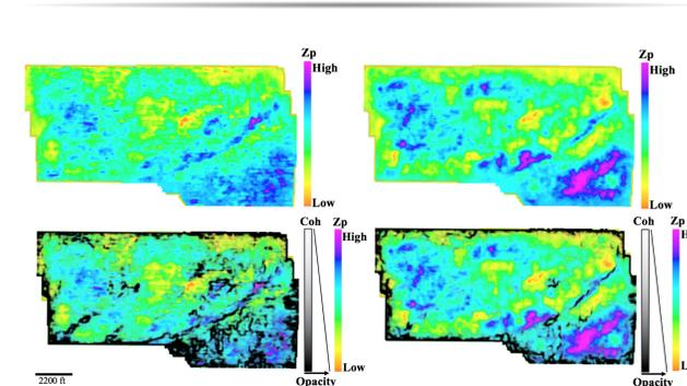
Figure 5: Top: Horizon slice along the top of the Mississippian through the P-wave impedance volumes obtained by prestack inversion of the original (left) and 5D interpolated data (right). Bottom: the same horizon slices through acoustic impedance co-rendered with coherence (a) before and (b) 5D interpolation.
