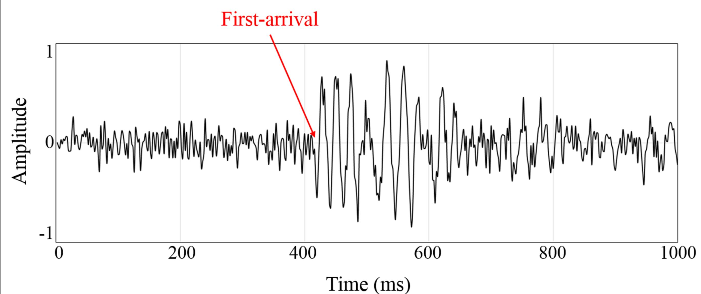
**Figure 1.** Micro-seismogram record. From this Micro-seismic trace, we can detect the first arrival that indicates by the red arrow.
