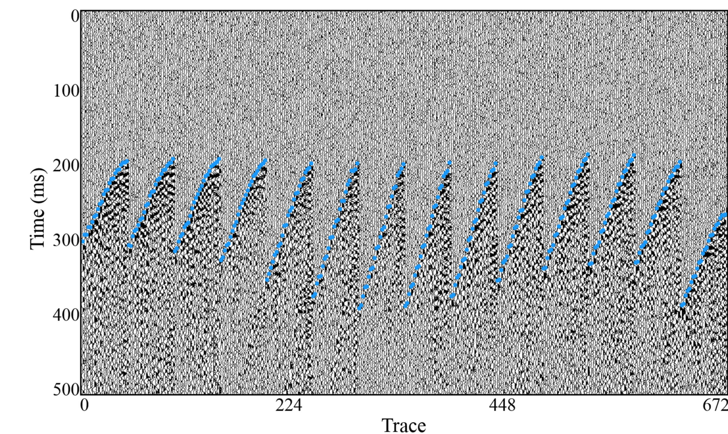
**Figure 6.** The field data example and the manually interpreted first arrivals (blue dots). We choose the first two gathers as our training data and rest as the test data.
