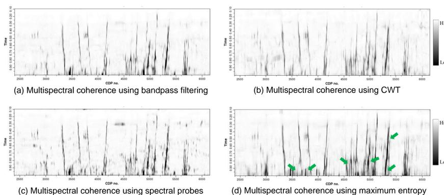
Figure 3: Multispectral coherence vertical slices using different spectral decomposition methods. Note the improvement of lateral resolution using maximum entropy method, highlighting small-scale discontinuities.
