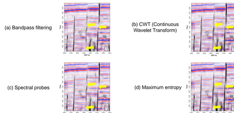
Figure 2: Maximum entropy based multispectral coherence provides the most continuous coherence image of the faults compared to other spectral decomposition methods
