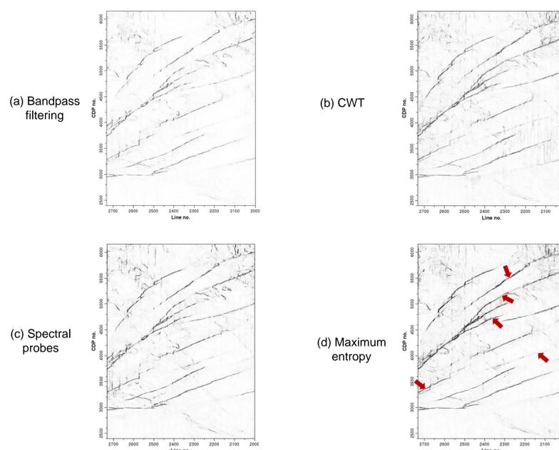
Figure 4: Multispectral coherence time slices (0.4s) using different spectral decomposition methods. Note the improvement of continuity of fault imaging using the maximum entropy method.
