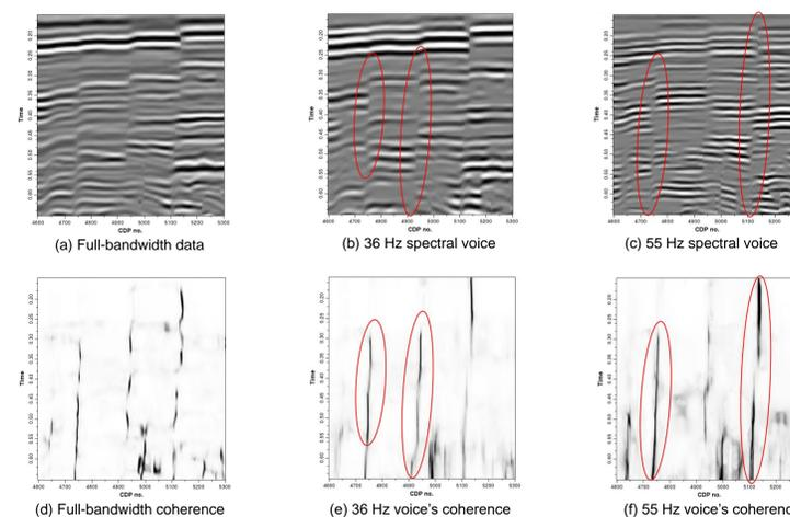
Figure 6: Coherence computed using full-bandwidth seismic data appears segmented due to the similar reflectors juxtaposing across the faults. However, because the phase is different for different spectral voices, alignment effects occur for only a few spectral voices not all components, which helps to fill the coherence gaps.
