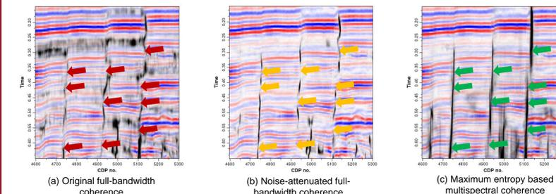
Figure 5: The full-bandwidth coherence computed using the noise-attenuated seismic data improves the quality of fault imaging over the original full-bandwidth coherence. Maximum entropy based multispectral coherence further improves the fault segmentations.
