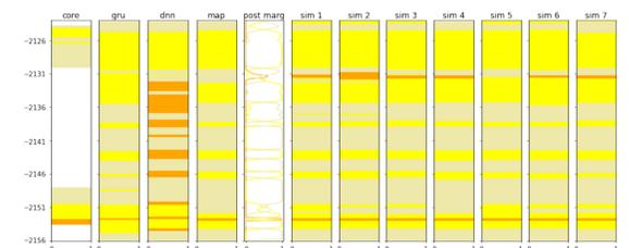
Figure 4: The comparison of the prediction results in the blind test well.
