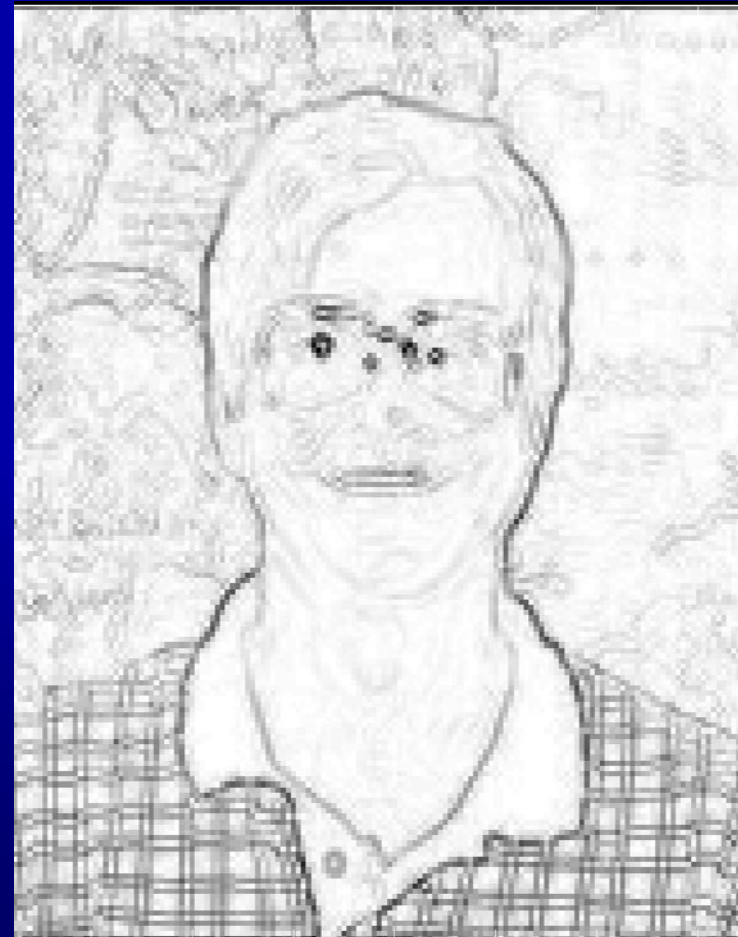
The Sobel filter: [(du/dx)^2 + (du/dy)^2]^{1/2}
